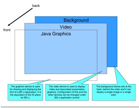
Figure 6-2 – BD-J system device model
