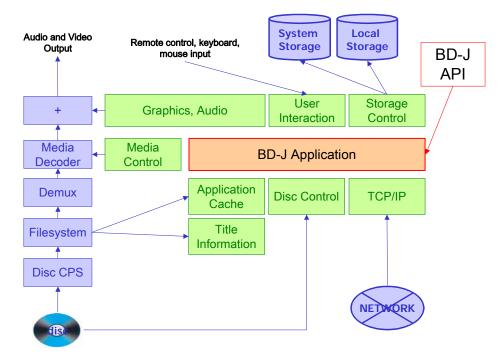
Figure 7-4 Interfaces between a BD-J application and BD-J System software
