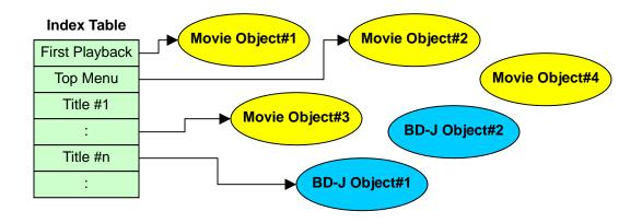
Figure 3-2 – An illustration of Index Table
