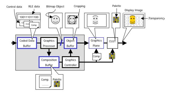
Figure 5-3 – Illustration of BD-ROM HDMV Graphics decoding
