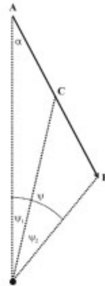
Figure 6 — The halfway point of the atmospheric trajectory does not divide the observed sky track into two equal angles.
