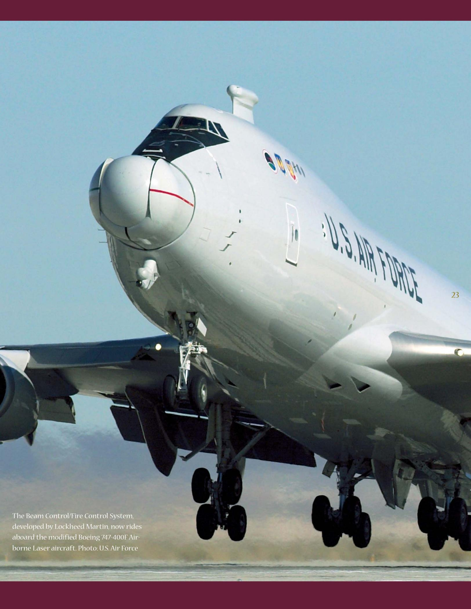
The Beam Control/Fire Control System, developed by Lockheed Martin, now rides aboard the modified Boeing 747-400F Airborne Laser aircraft. Photo: U.S. Air Force
