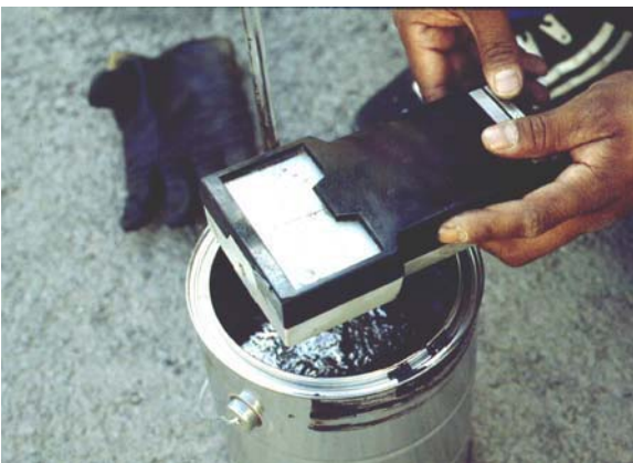
Figure 3-7: Hand Held Viscometer Testing
