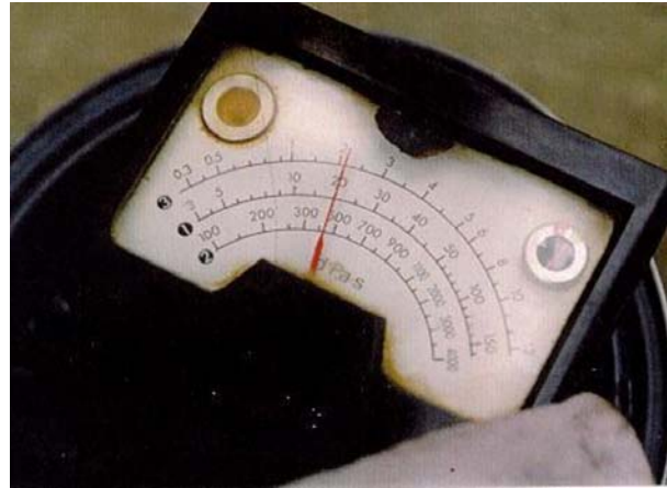
Figure 3-8: Viscometer Reading—Scale No. 1
