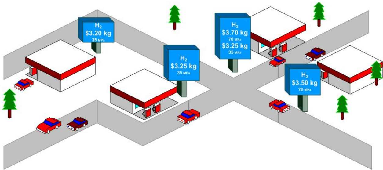
Figure 3. Showing the Use of the Uniform Unit of Measurement and Posting of Service Pressure in MPa to Enable Value Comparison
