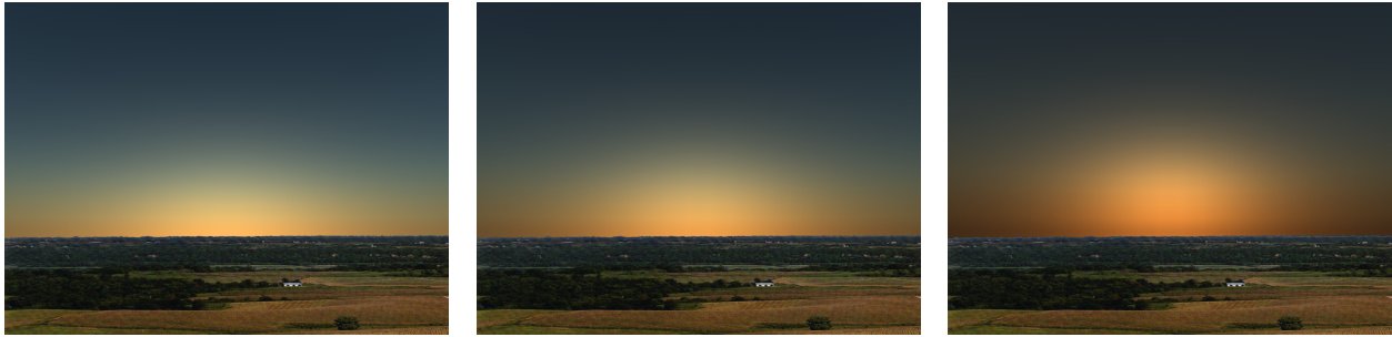
Fig. 8. Effect of varying humidity on the colors of the sky. Left to right: 50%, 80%, and 95% humidity. All simulations have been performed for the same location, time (6:35 pm DST, sun elevation +9^\circ ), and type of climate (continental, average pollution).
