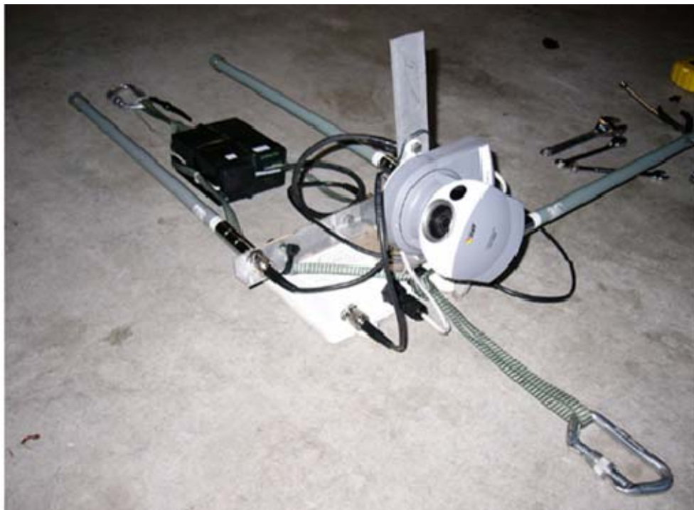
Figure 24. Completely assembled payload with camera
