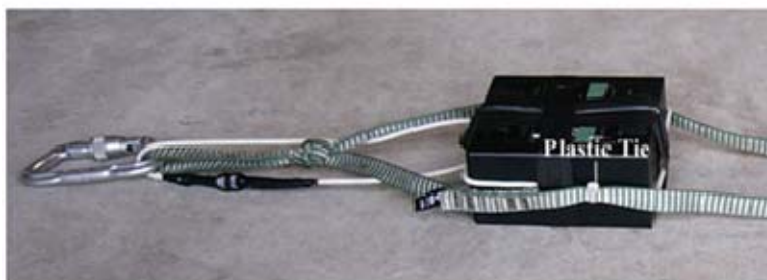
Figure 17. UBI-2590 Battery secured on sling
