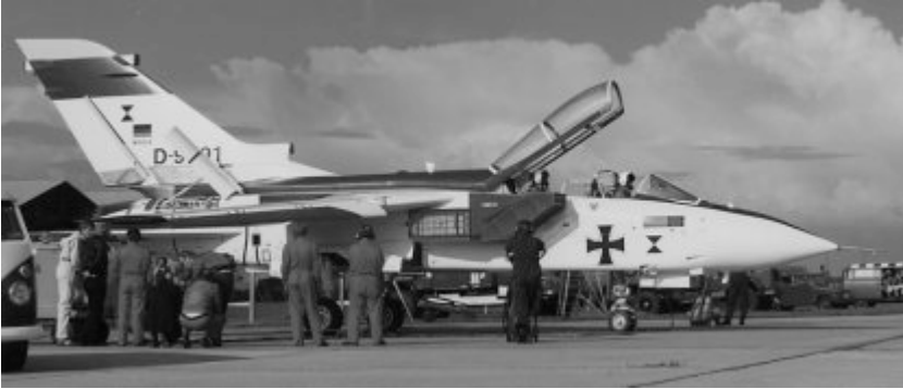
Engine runs on P01 at Manching prior to first flight.
