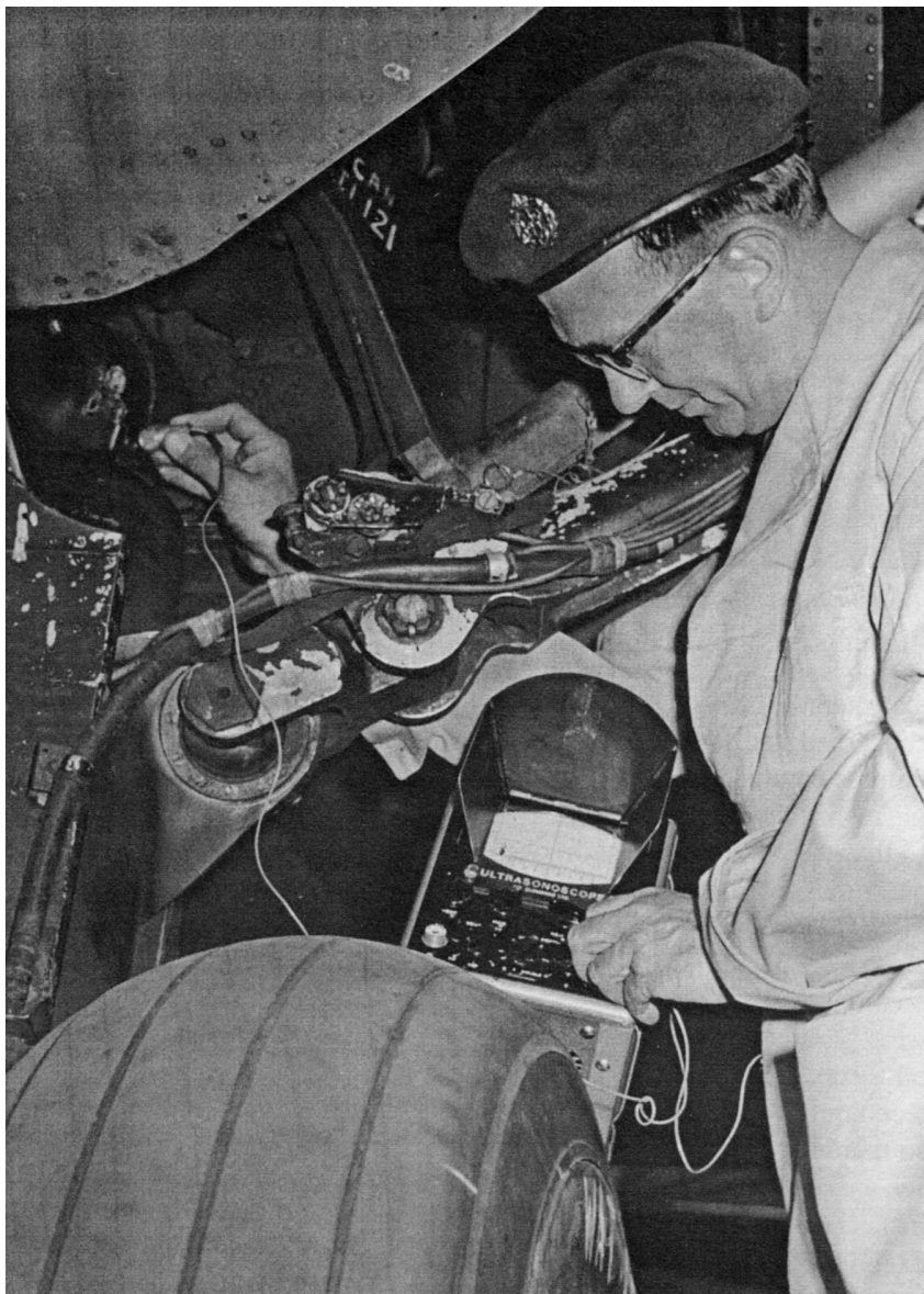
Carrying out an ultrasonic inspection on the undercarriage of a Canberra.
