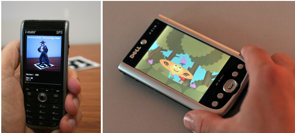
Figure 2.5: Left the screen of the handheld represents the AR display; Right: the handheld itself represents the AR display.
