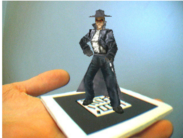
Figure 4.2: Textured avatar "Caleb" rendered on top of an ARToolKit fiducial marker using Klimt.
