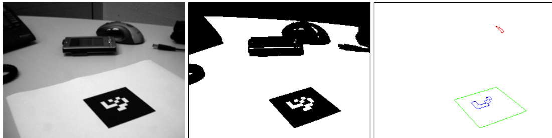
Figure 3.4: Fiducial Detection in ARToolKitPlus. Left: Source image; Middle: Threshold image; Right: Three closed polygons as candidates for rectangle fitting.
