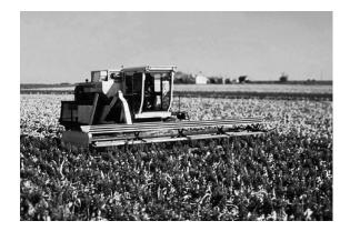
According to Kevin Bien, product marketing manager for GLEANER combines, the transverse-flow fan and electro-hydraulic controls were both new concepts in the industry. So was torque-sensing drive, which also made its debut in 1972.
