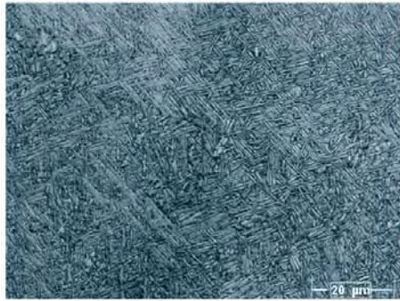
Figure 4.7: Microstructure of the melting zone of a laser build-up weld of the titanium alloy Ti624.
