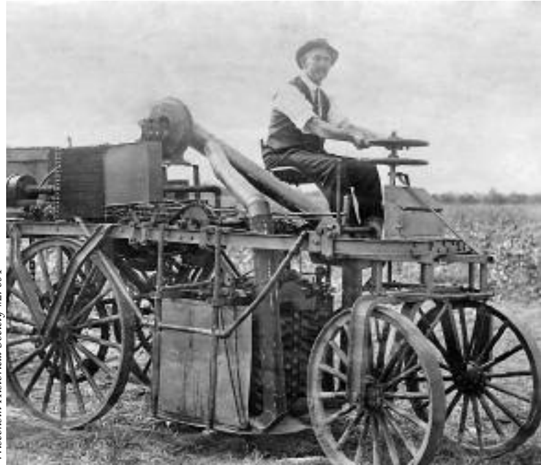
One of the first spindle-type cotton pickers, a 1924 Price-Campbell.
