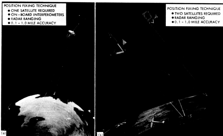
Figure 19.—Navigation satellite concepts. (a) Range-angle-angle; (b) range-range.
