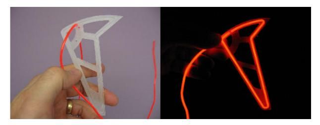
Make it easy to see the orientation of your night heli with these high quality Lexan fins specially designed with a slot for cold light strings. (Light strings not included)
