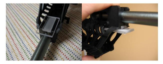
This device allows you to mount your gyro inverted to protect it against blade or paddle strikes. It is made of high quality Lexan and machined to proper dimensions. It comes with high strength mounting tape.
