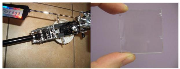
This mount provides a rigid mounting surface for your gyro or receiver. (Designed by helifreak BobOD). It is made of high quality Lexan and machined to proper dimensions.
