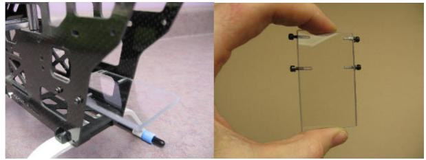
This mount provides an additional rigid mounting surface for your gyro, receiver, or both. (Inspired by Helifreak ChasHeliCop). It is made of high quality Lexan and machined to proper dimensions. It comes with four M2x8 screws included.
