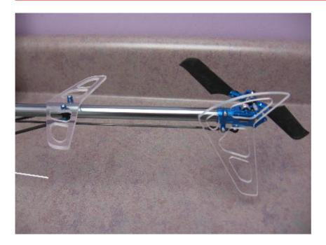
Stop breaking your stock fins and tail blades. These Lexan fins are sturdier than the stock CF fins, and they are longer to better protect your tail blades. Both the Horizontal and Vertical fins come pre-drilled and ready to install. Longer screws may be required.
