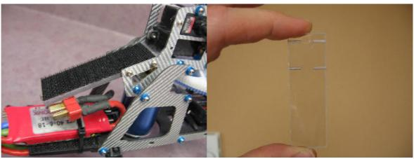
This mount provides a secure but flexible mounting surface for your battery. (Inspired by Helifreak copterklutz). It is made of high quality Lexan and machined to proper dimensions.
