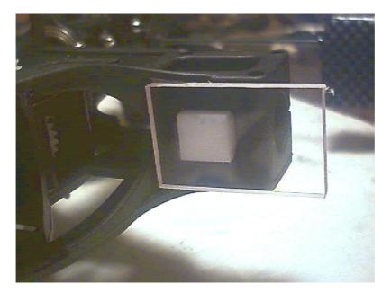
This device allows you to mount your gyro inverted to protect it against blade or paddle strikes. It is made of high quality Lexan and machined to proper dimensions.
