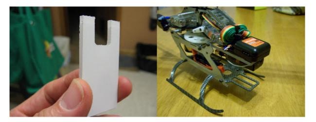
This mount gives you more room for mounting your receiver and/or your gyro. (Inspired by Helifreak user BuzzKill). It is made of high quality Lexan and machined to proper dimensions. It mounts with the hardware that came with your 200.
