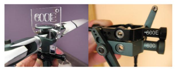
T-REX Original Design Flybar Locks: These tools lock your flybar firmly in place while you adjust your pitch ranges. Lexan tool won't scratch your paint. These locks do not require a head button.
