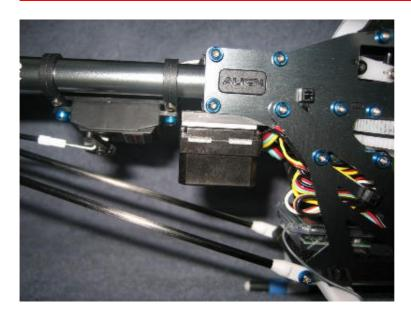
This device allows you to mount your gyro inverted to protect it against blade or paddle strikes. It is made of high quality Lexan and machined to proper dimensions. This is for the XL Carbon Frame upgrade with the plastic boom block or the SA which has a plastic boom block.
