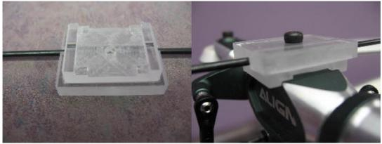
This tool mounts on top the head to provide a level reference for your pitch gauge to allow accurate blade pitch adjustments on Flybarless heads. (Inspired by Helifreak caralmar). A TREX 450 Flybar is used as reference bar (not included). Attaches with stock button screw (not included). Lexan tool won't scratch your paint.
