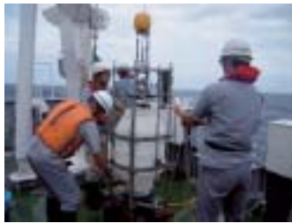
Sampling of seawater in radioactivity research
