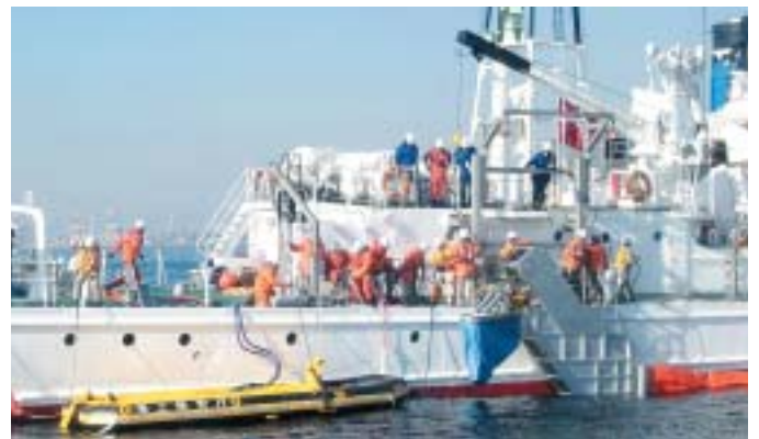
Oil recovery equipment for high viscosity oil (LSC)
