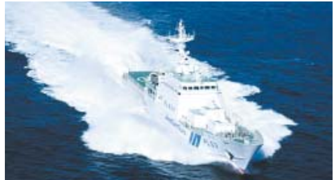
2,000-ton patrol vessel (high-speed / high-performance, helicopter-carrying-type) Kiso commissioned to track suspicious ships
