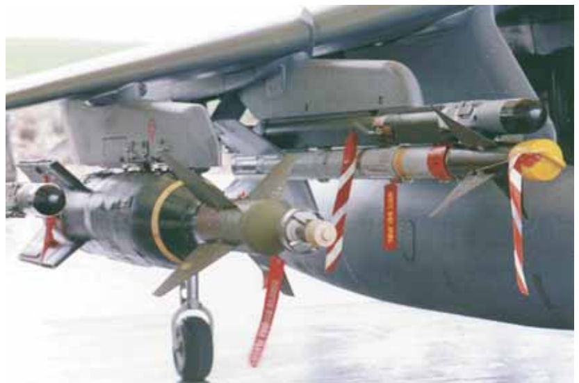
A Paveway II LGB under the wing of a Harrier GR7 aircraft
