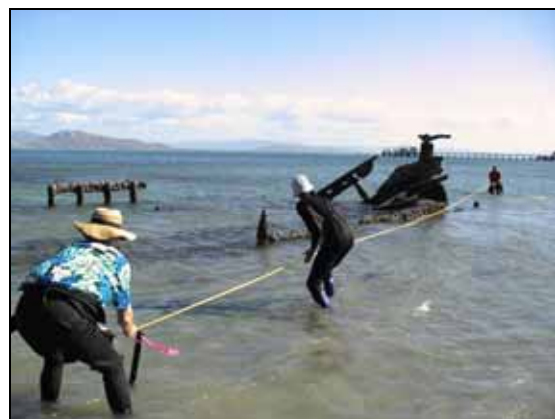
(Trilateration mapping on the remains of George Rennie . Image: James Cook University)
