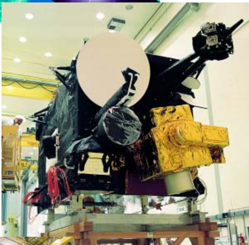
Above: unpacking the Flight Model after its arrival at ESTEC to begin systems-level testing in July 1998. The SILEX terminal is at bottom right; the telescope is pointing down. Above it is the Ku-band feeder link for the LLM land mobile package. At top left is the Ka-band feeder for the SKDR and SILEX packages.
