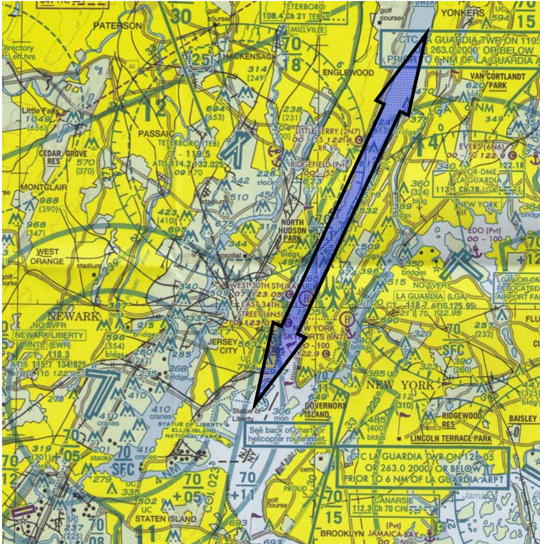
Figure. New York VFR Terminal Area Chart depicting class B boundaries, shown as blue lines. The large blue arrow marks the Hudson River class B exclusion area.
