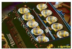
Formula One of the time. Engine length, weight and stiffness were cited as main concerns and Dudot used this information to decide on the V10. This was not a natural engine layout due to the harmonics of the odd firing order and crank shaft timing. But the V10 would be a larger but more powerful engine than the V8 Ford was still running, but shorter than the V12, despite less power potential.
