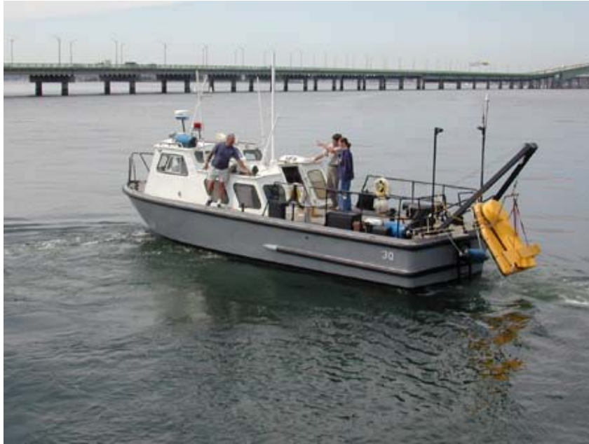
Fig 13 US Navy Workboat 30 preparing to deploy the Sub-bottom Profiler off the Newport - Jamestown Bridge. Photo K. Hosty.
