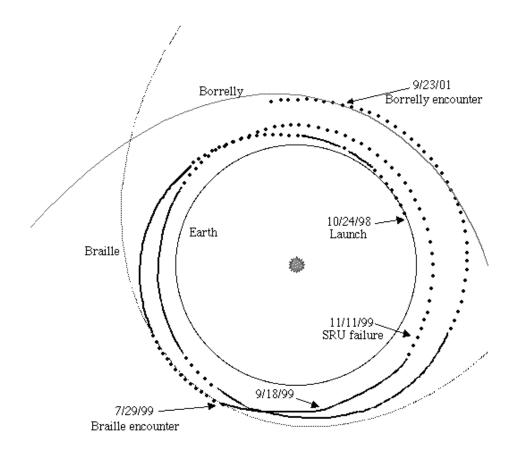
Figure 1. DS1 trajectory for the primary mission (through September 18, 1999) and extended mission. The dotted portion is for ballistic coast; the solid portion indicates the IPS is used for deterministic thrusting. As explained in the text, the IPS is on (in some cases at very low throttle levels) for most of the mission after the resumption of thrusting following the SRU failure.
