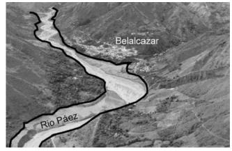
**Fig. 7.** Effects of the 1994 debris flow from Nevado del Huila in the Páez river at the town of Belalcázar, where flow heights reached over 20 m. Trimlines of the 1994 flow are indicated. (Photograph courtesy of H. Cepeda.)
