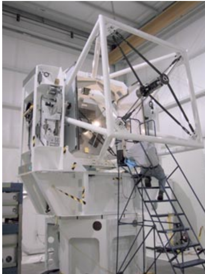
Figure 3: 2m tracking telescope specifically developed for debris tracking. It has diffraction-limited optics and servo systems with similar limits [EOS image].
