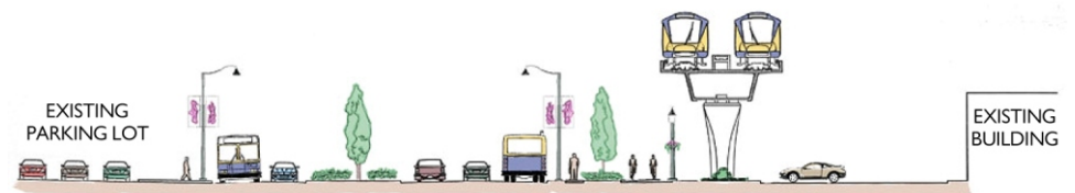
Example of elevated guideway on No. 3 Road
