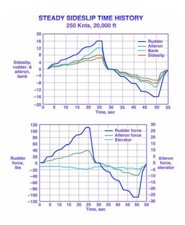
The recorded data from a Steady Sideslip is shown in Fig. SS-8.
