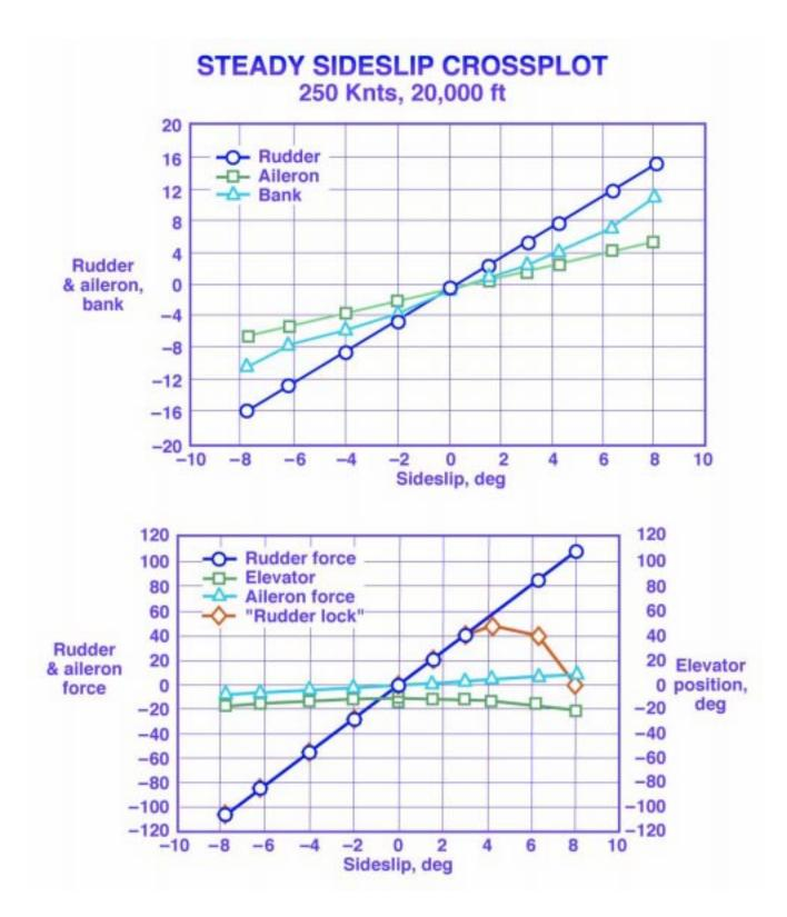
Any nonlinear tendencies in the rudder force gradients (that is, lower rudder forces needed at the higher rudder deflections) will be carefully reviewed. If a rudder lock condition is suspected, a repeat maneuver, or an additional maneuver at a slightly different flight condition, might be flown.
