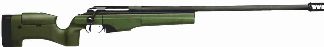
SAKO TRG based on a series of actions which designated: Short action TRG-22 and Long action TRG-42. Receiver is made by coldhammering method. Three locking lugs makes 60° bolt lift angle possible. The receiver is stabilized with three fastening screws. Optionally available with phosphatized finish. The bolt is black matte on all models.
