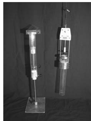
The sediment corer used in the lake survey.
