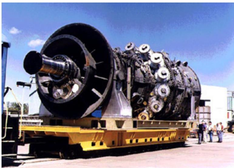
Figure 14: First MS9001H gas turbine at GE's facilities (Greenville, SC).
