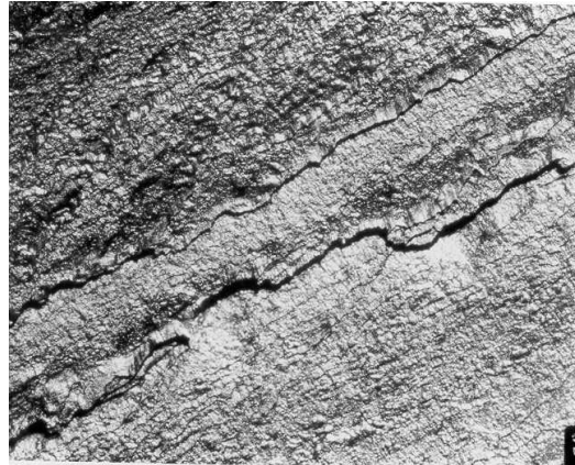
Figure 9: Surface Tears Preform ~ 13X.
