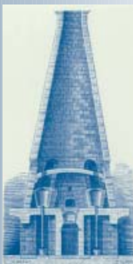
Figure 7: William Champion's zinc smelting furnace.
