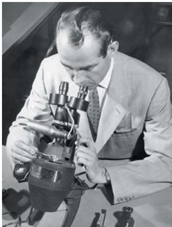
Figure 4. During his several decades in the laboratory, Bob Crowningshield used the microscope for many of his discoveries. This photograph, taken in the 1950s, shows him using an early-version Diamondscope, a binocular gemological microscope with lightfield and darkfield illumination that had been developed by GIA in the 1930s and '40s.
