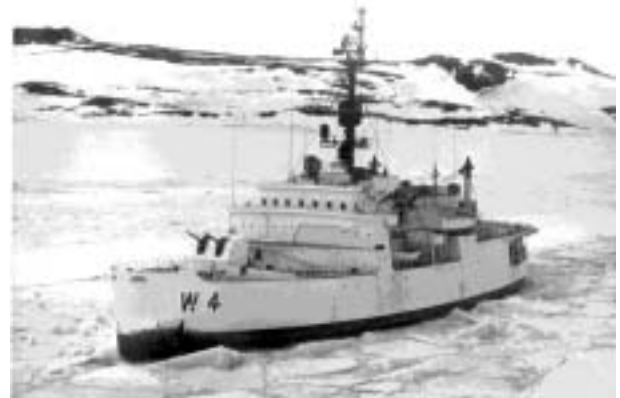
USCGC Glacier clears a channel for McMurdo Station. Due to her high hull strength and propulsion power, Glacier was able to open up areas in the Antarctic and Arctic previously inaccessible to navigation. Glacier can break ice 4 feet thick continuously at 3 knots. (USCG Photo)
