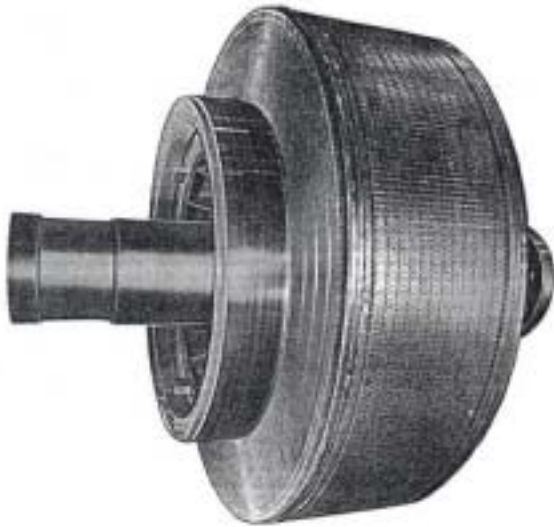
A flange is forged on the aft shaft extension of the propulsion motor armature (to the right in figure) for direct coupling to the propeller shafting. Each propeller weighs 17 tons. (Westinghouse Photo)
