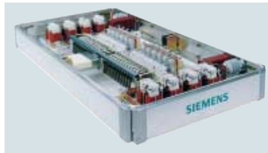
Fig. 5.1-4: Valve module with direct-light-triggered thyristor
