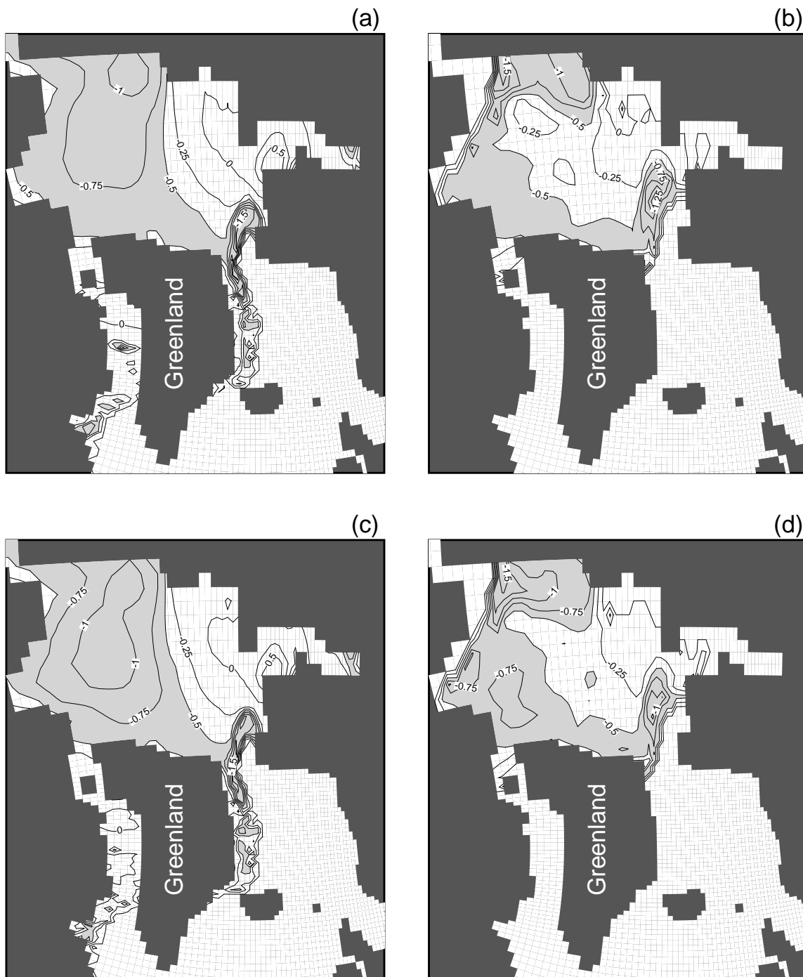
Figure 3.11: Changes in the simulated ice thickness (m) after 20 years in (a) March, (b) September, and after 90 years in (c) March and (d) September. Contour intervals: 0.25 K, shaded area = ice thickness reduction > 0.5 m.
