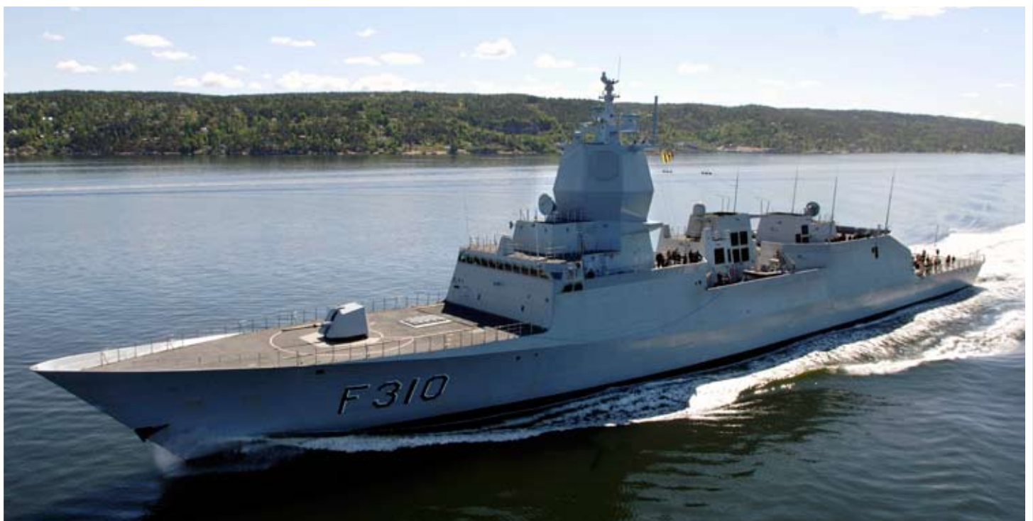
Flexible. The Nansen class frigates are the backbone of Norway's future naval defense. The frigates will have the capability of combating submarines, surface vessels and air targets. Each of the frigates will have a NH-90 helicopter on board. (Photo: FMS)
