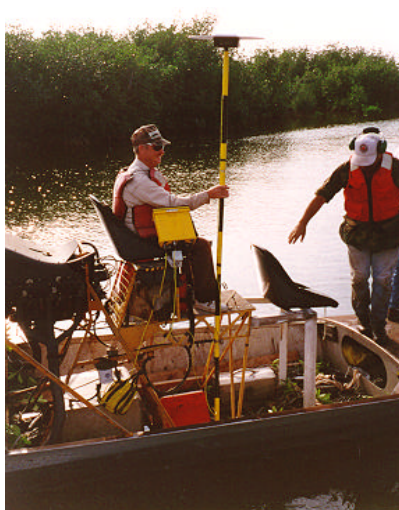
Figure 6-4. GPS RTK surveys from airboat operating in shallow wetland areas (Jacksonville District)
