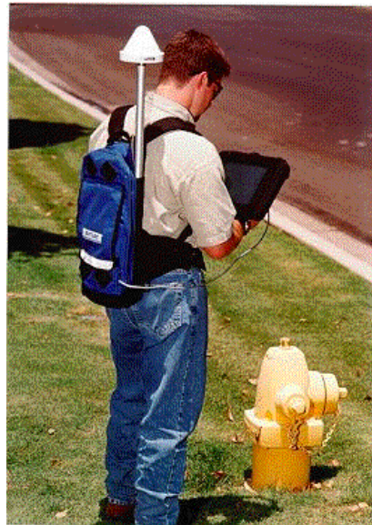
Figure 9-8. Real-time, meter-level accuracy, feature mapping-grade GPS backpack systems
