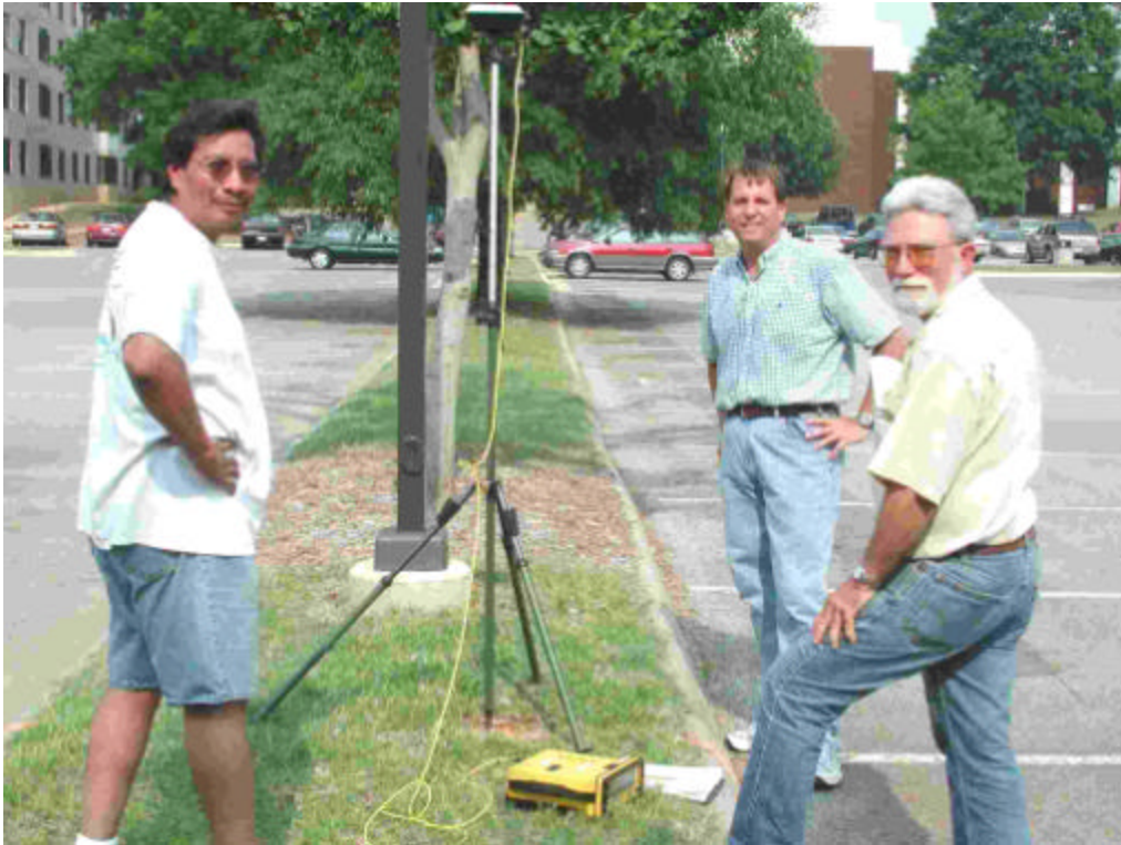
Figure 6-2. Fast-Static control survey of topographic reference monument at Huntsville Bevill Center
