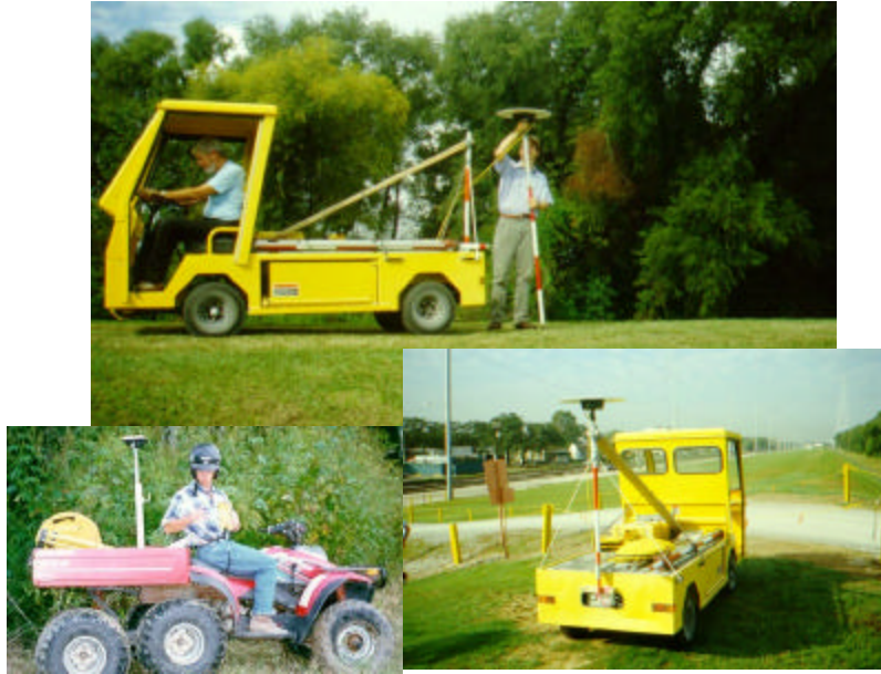
Figure 6-5. New Orleans District levee profiling using real-time kinematic GPS methods (New Orleans District and 3001, Inc.)
