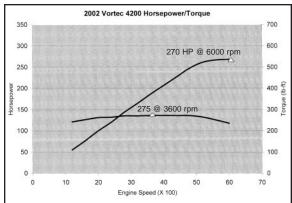
The Vortec 4200's torque curve extends through the majority of the speed range. Ninety percent of the peak torque is available from 1,600 to 5,600 rpm.
