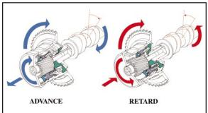
The valve timing is electronically controlled and solenoid actuated by advancing the exhaust cam relative to the intake. Very little exhaust gas is allowed into the intake charge. The result is a smooth and clean combustion that enables good torque and power throughout the speed range and reduced emissions.
