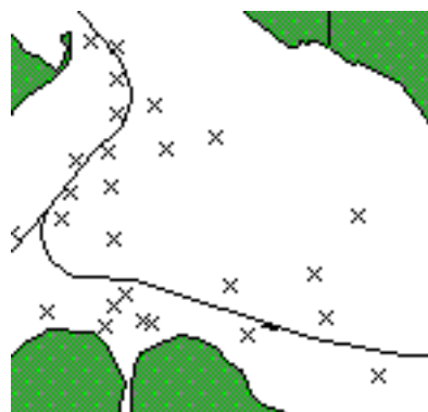
Figure 3: The first two curves in the channel leading up to Southampton harbor. The line indicated the planned course; crosses equals buoys.
