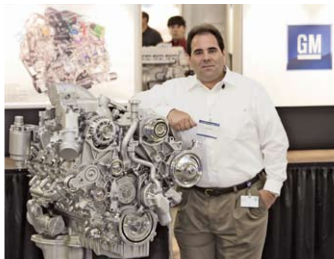
GM’s Gary Arvan flanks the automaker’s 2007 Duramax 6.6-L turbocharged diesel engine, which uses a revised E35 controller with new control software to meet emissions requirements.
