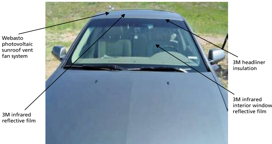
The NREL's retrofitted STS demonstrated how reducing passenger-cabin heat gain and venting hot-soak air would permit use of a smaller-capacity A/C system.
