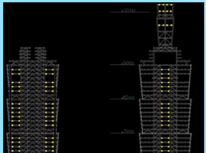
Figure 10: Yellow dots show locations of Reduced Beam Section 'dogbone' details for enhanced ductility at points of greatest flexural rotation demand.
