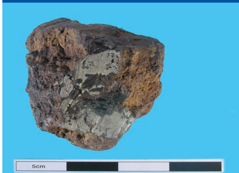
Fig. 2: Side view of the Trewiddle bloom, showing the surface freshly exposed from this study.
