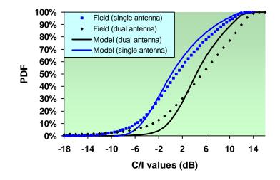
Figure 3. The C/I probability distribution function from simulations and measurements.
