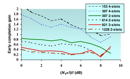
**Figure 9.** Early completion gain as a function of (N<sub>0</sub>+I)/I. N<sub>0</sub>—Noise density I—Interference density
