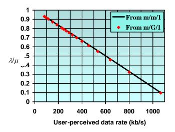
**Figure 13.**  $\lambda/\mu$  based on the 3GPP2 FTP traffic model.
