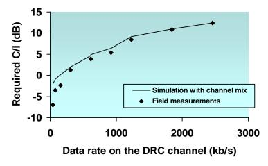
Figure 7. The required C/I derived from measurements and simulation.
