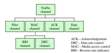
Figure 1. Reverse link traffic channel structure.
