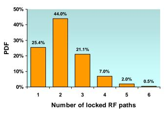
**Figure 4. Number of locked RF paths for the demodulator.** PDF—Probability distribution function
