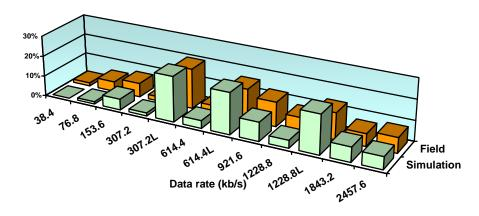
Figure 5. Distribution of the data rate on the DRC channel.
