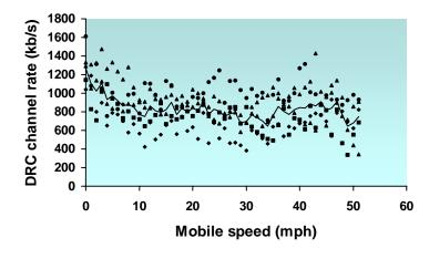
Figure 6. Data rate measured on the DRC channel as a function of speed.
