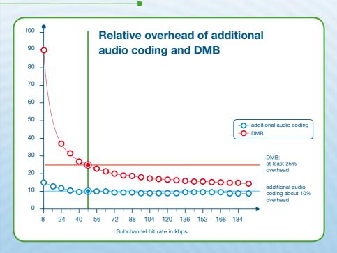
This figure shows a comparison of the relative overhead (used for error correction and transport protocol) of additional audio coding (assuming no PAD information) and DMB (PAD information not possible) in case of a radio service.
