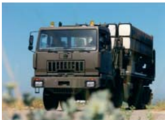
SAMP/T Block 1 batteries (12 French and 6 Italian) are characterised by a high strategic mobility thanks to their air portability by C-130 Hercules; as well as tactical mobility due to the reduced staff and vehicles needed for their positioning. Launchers are fitted on highly mobile 16 tons trucks. Shown above, an Italian 8x8 Iveco. (MBDA).
