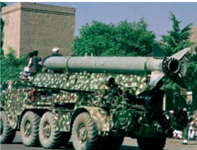
A Frog-7, ground-to-ground artillery rocket, of 65 km range, in the streets of Kabul, Afghanistan. (AFP)
