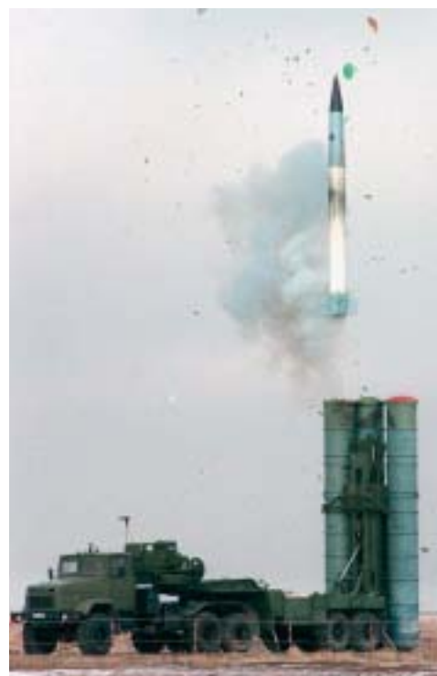
Quadruple launcher on a SA-10 Grumble truck (S-300 PMU). Shown above is the modernised version, called S-400 by its manufacturer Almaz ; undergoing tests in the Kasputin Yar centre, near Astrakhan in February 1999. (AFP)
