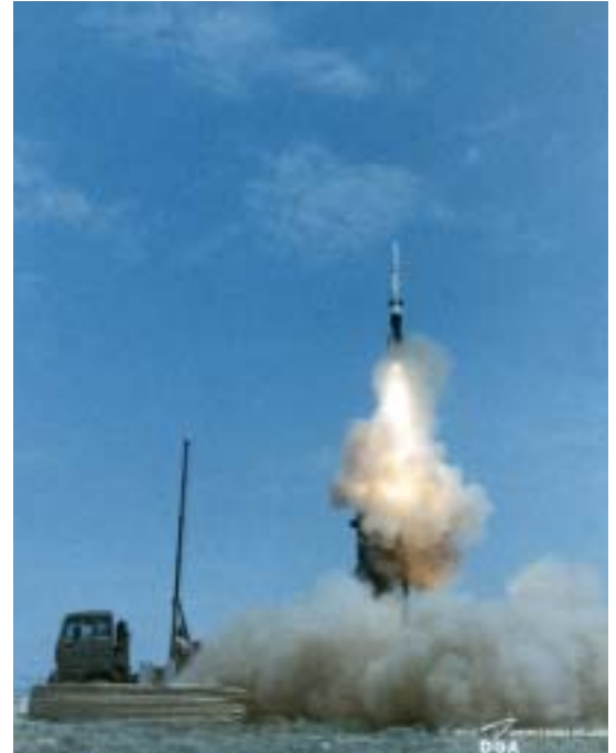
When entered into service in 2005, SAMP/T, based on the Terrestrial Aster 30 missile, will be the first European system capable of intercepting a Scud of 300 km range as well as the Super-Scud (600 km range). ATBM configuration of the Terrestrial Aster 30, known as "Block 1", has been settled in a development contract between France and Italy in May 2000. (DGA/CEL).
