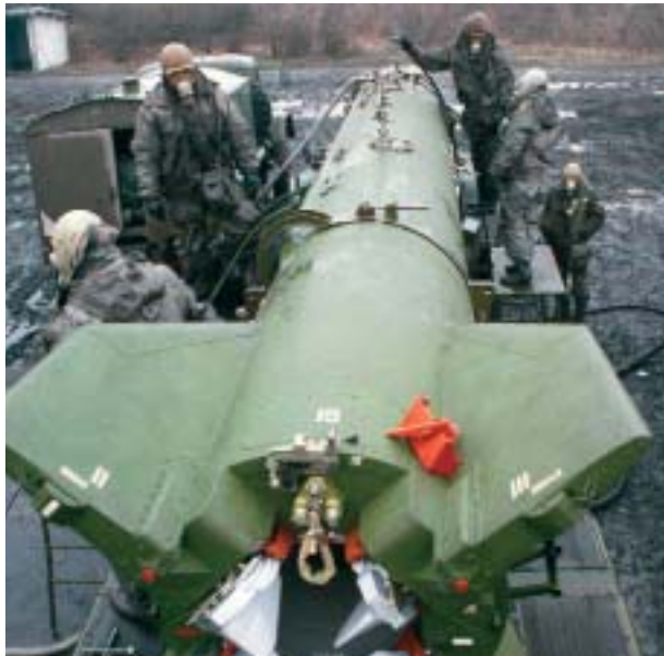
Rear view of a Russian Scud B, with details of the deflectors (silver coloured graphite) which are used for missile piloting ; the drift (in green) are fixed. (AFP)
