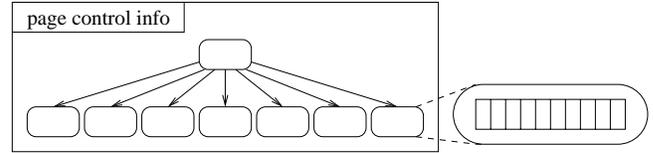
Figure 5: Disk-first fpB<sup>+</sup>-Tree: a cache-optimized tree inside each page
