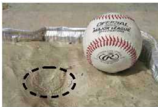
Figure 5.5: A regulation baseball and a crater of its impact. Pitching machines threw baseballs at tubs of Plumber's Putty. A chronograph measured the speed of each baseball. The baseball speeds were approximately 40, 50, 60, 70, 80, and 90 miles per hour.
