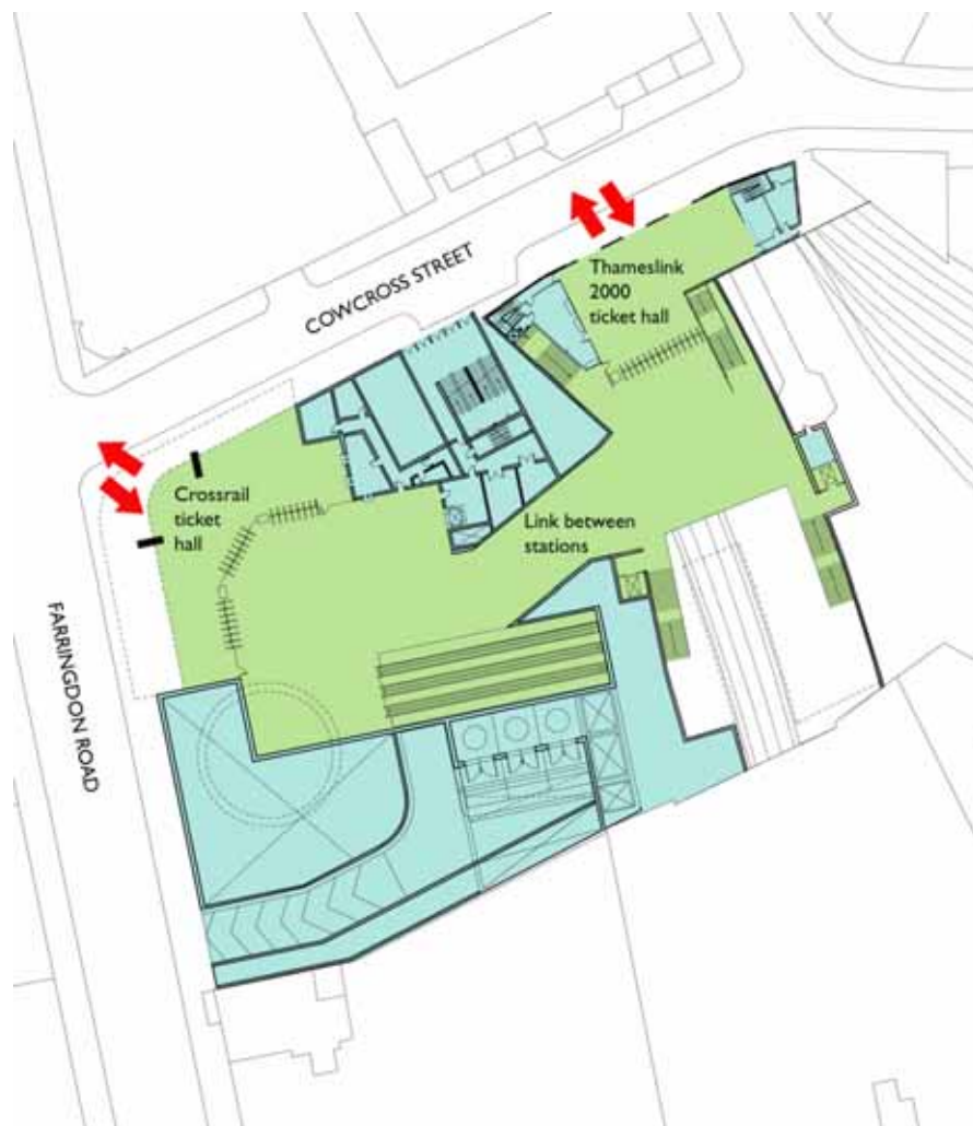
Figure 2.9 (ii): Interchange at Farringdon between Thameslink 2000 station and Crossrail station (western ticket hall)
