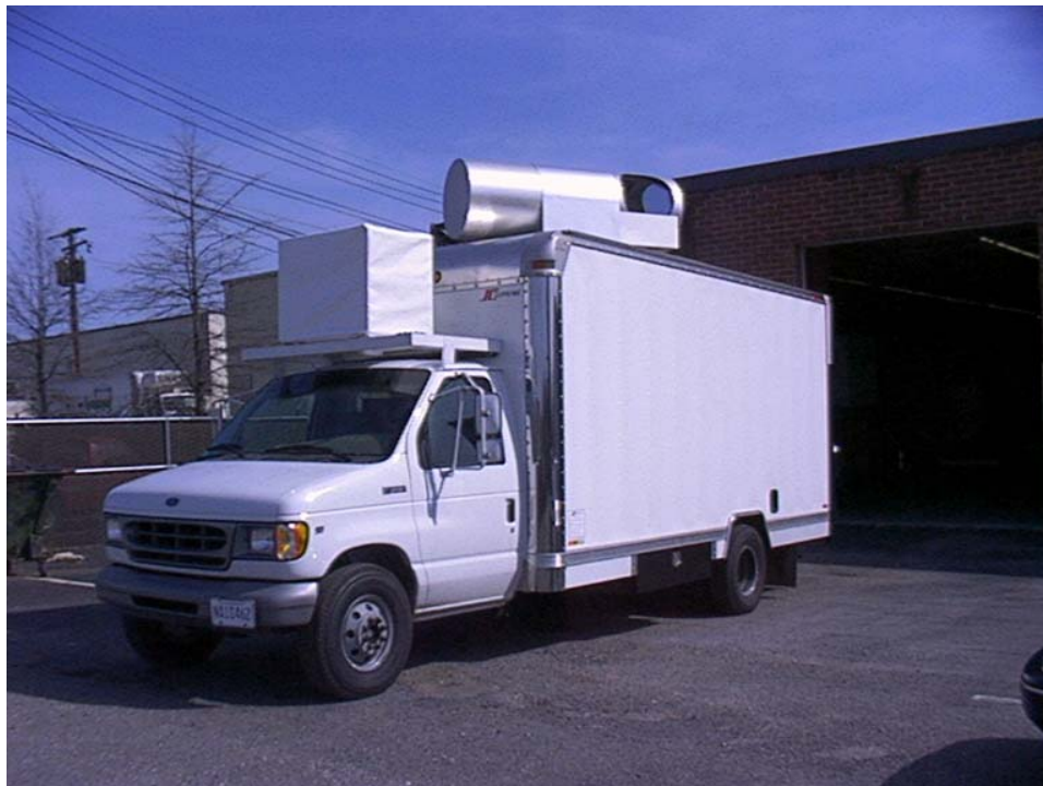
Fig. 7. GLOW lidar in mobile van at NASA-Goddard Space Flight Center.
